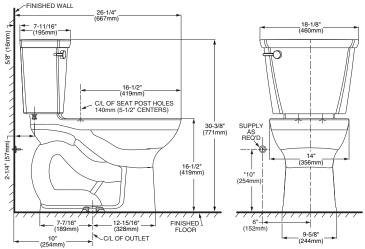
THIS TOILET IS DESIGNED TO ROUGH-IN AT A MINIMUM DIMENSION OF 254MM (10") FROM FINISHED WALL TO C/L OF OUTLET.
